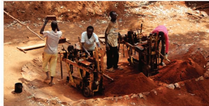
the production of CEB blocks on site
